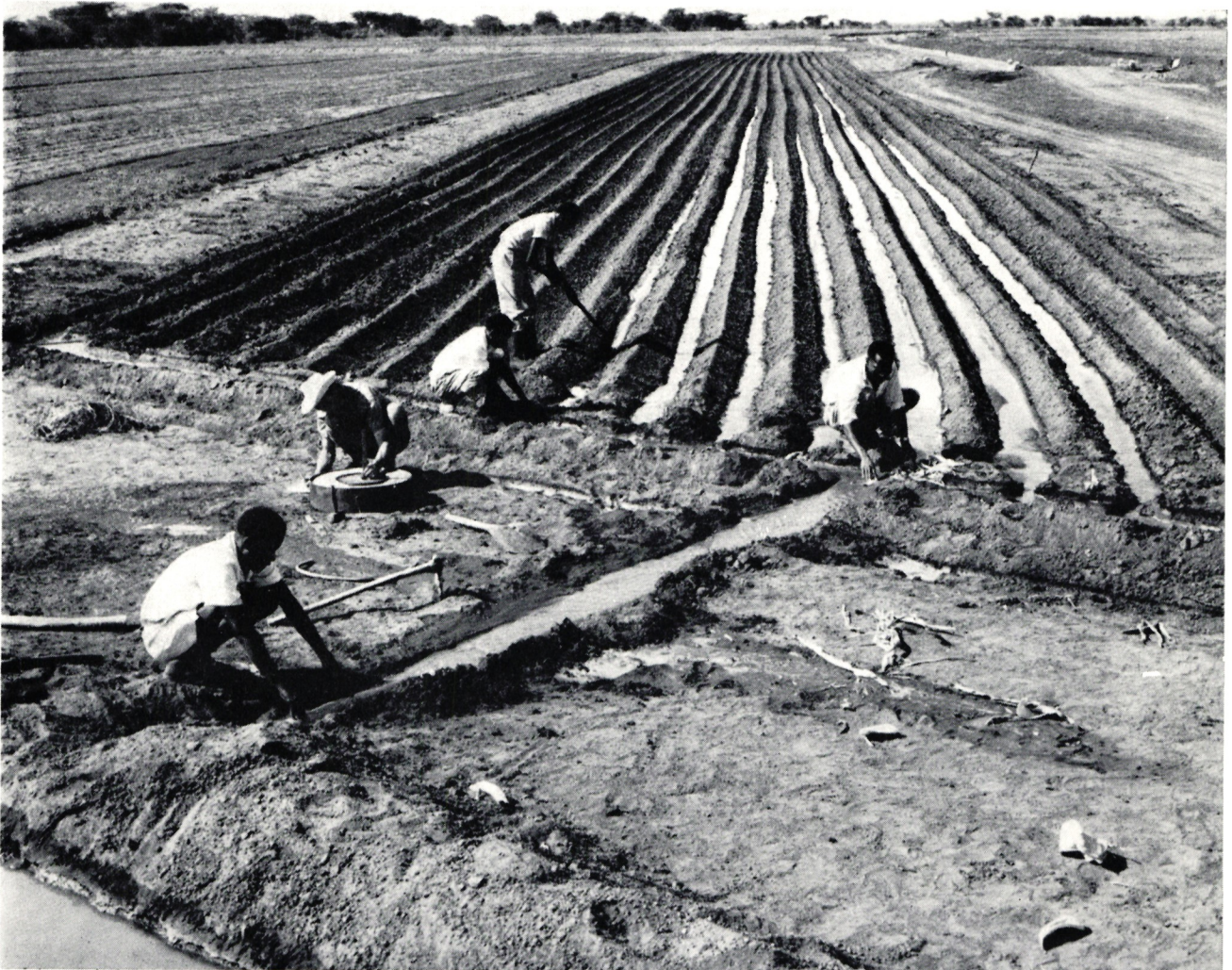
Fig. 8.—PERKERRA IRRIGATION SCHEME.—Infiltration tests and furrow application trials in progress.
