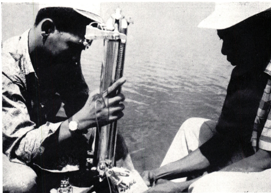
Fig. 6.—ISOTOPE INVESTIGATION OF THE HYDROLOGY OF LAKE CHAKA. Sampling the lake water for Tritium Concentration.
